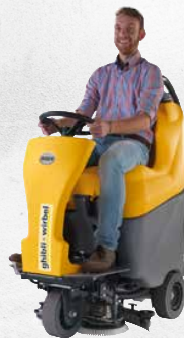
RIDER R 65 FD 65 Four brushes, cleaning width 650 mm, squeegee width 750 mm
